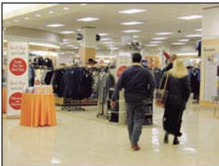
Spot the exit sign – 'Exit signs must be clearly visible at all times'. The one in this picture is larger than required and about 50 metres away – the proposed maximum distance allowed between signs
